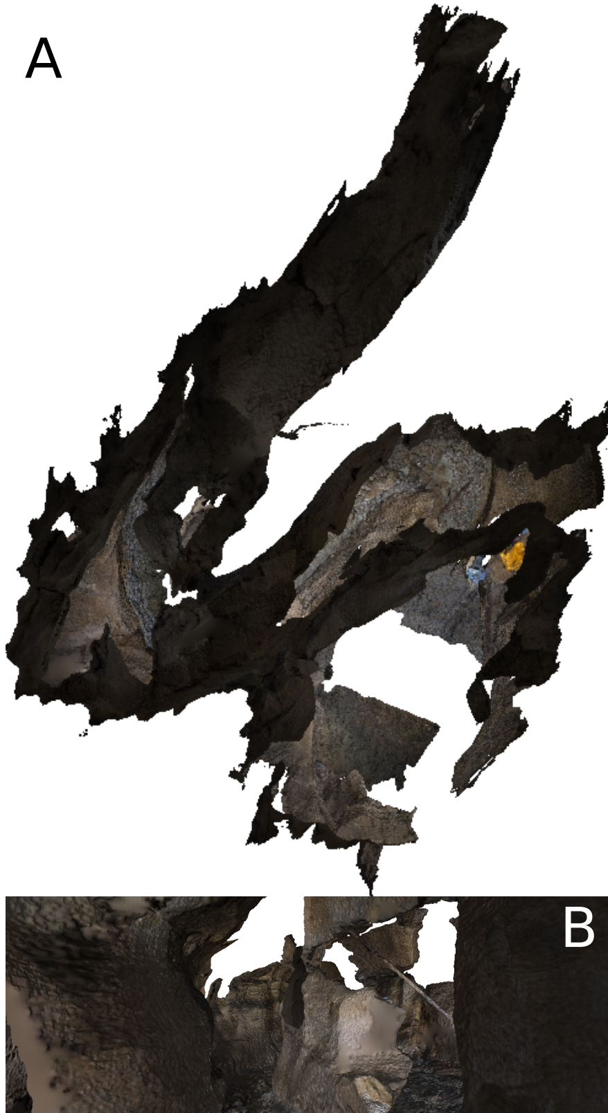
Figure 2: (A) 3D model plan view of an area in Gourdneck Cave. (B) A view into the model towards the closed loop in the scan.
